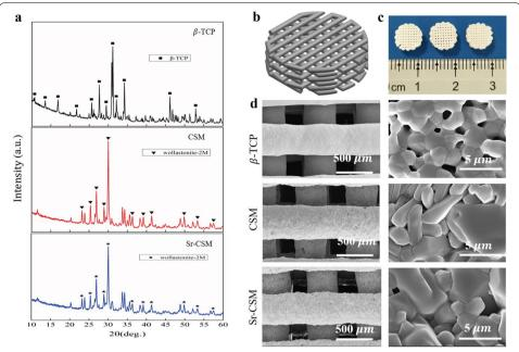
**Fig. 2** Characterization of the β-TCP, CSM and Sr-CSM powders and scaffolds. **a** XRD patterns of three bioceramic scaffolds, **b** CAD model of three bioceramic scaffolds, **c** digital photograph of three bioceramic scaffolds: from left to right is β-TCP, CSM and Sr-CSM, **d** SEM images of three bioceramic scaffolds
