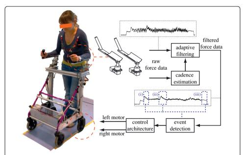
**Figure 11 Complete system architecture implemented in the SIMBIOSIS walker's firmware**. The output signals of the filtering architecture presented in this paper is used by a event detection algorithm that classify the signals in real-time and send navigational commands to the controller that commands directly the walker's dc motors. For illustration purposes, three areas are distinguish with blue boxes: (i) start walking, (ii) right turn and (iii) stop walking.
