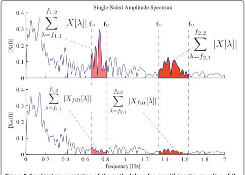
**Figure 9** Graphical representation of the methodology for quantifying the canceling of the cadence related components of force data. *R* indicates the reduction of signal's energy within the cancelation range given by the frequency input of the FLC algorithm presented in this work.
