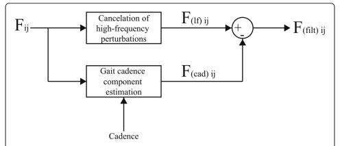
**Figure 3 Signal processing architecture for user's intent component separation.**  $F_{ij}$  is the force signal obtained from axis (j), sensor (i).  $F_{(tf)_{ij}}$  denotes the force signal obtained after the high frequency noise cancelation and  $F_{(cad)_{ij}}$  is the periodical, cadence-dependent component of force. Finally,  $F_{(filt)_{ij}}$  is the processed final signal related to user's navigation intent.
