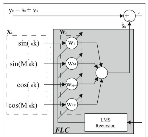
**Figure 5 The Fourier Linear Combiner algorithm**. The adaptation of the coefficients  $w_k$  is performed based on the least-mean-square (LMS) recursion.  $y_k$  is the input signal. The adaptive weight vector,  $\mathbf{W}_k$ , generates a linear combination of the harmonic orthogonal sinusoidal components of the reference input vector,  $\mathbf{X}_k$ . M is the number of the harmonics used and  $\mu$  represents the amplitude adaptation gain used for the LMS recursion.
