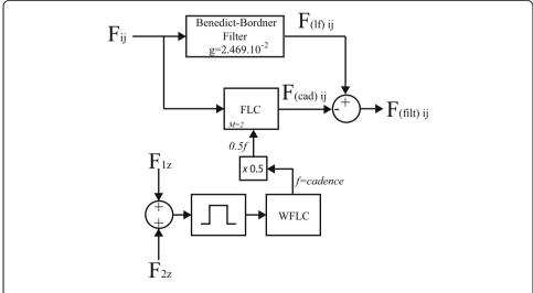
Figure 7 Final signal processing architecture for estimation of user's intent force component considering the possibility of asymmetrical supporting forces.
