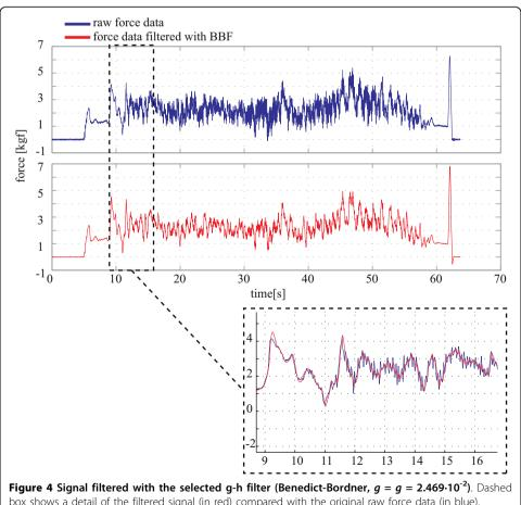
box shows a detail of the filtered signal (in red) compared with the original raw force data (in blue).
