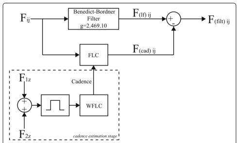
**Figure 6 Signal processing architecture for estimation of user's intent force component.**  $F_{ij}$  is the force signal obtained from axis (j), sensor (i). F(if)ij denotes the force signal obtained after the high frequency noise cancelation and F(cad)ij is the periodical, cadence-dependent component of force. Cadence estimation stage by means of WLFC is indicated with dashed lines.
