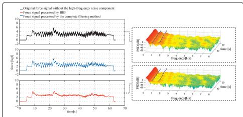
Figure 10 On the left, representation of force data for the y axis of the left sensor in one experiment in three stages: raw force data (top), data after the BBF (middle) and final output (bottom). On the right, the spectrogram of the filtering input (top) and output (bottom) are presented along with the continuous line marking the continuous cadence estimation by means of WFLC. Important reductions in PSD of high frequencies and in both cadence harmonics are observed.
