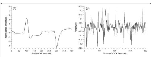
**Figure 4 A preprocessed two-lead heartbeat and its ICA features. (a)** A preprocessed LBBB heartbeat. **(b)** The ICA features of the heartbeat shown in (a).
