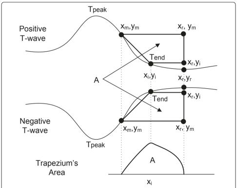
Figure 3 Determination of the T-wave end (for a monophasic wave) by the computation of the areas of several trapezes formed by three fixed points and one mobile  $(x_i, y_i)$ . The Tend corresponds to the point where the area A is maximum.
