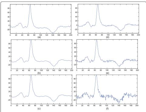
**Figure 6** Example of a beat of QTDB (from sel32 recording, first channel) with different levels of noise: (a) Original beat, (b) Band-pass filtered version of (a), (c) 3 of noise of  $A_{TWP}$ , (d) 5% of noise of  $A_{TWP}$ , (e) 10% of noise of  $A_{TWP}$  and (f) 20% of noise of  $A_{TWP}$ .
