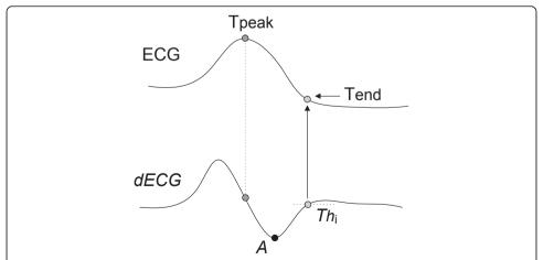
**Figure 2** Threshold method on the first derivative applied to a positive T-wave. A threshold for the i-beat ( $Th_i$ ) is calculated by dividing the minimum derivative value by an empirical factor (K). The first sample below  $Th_i$  is defined as the T-wave end.
