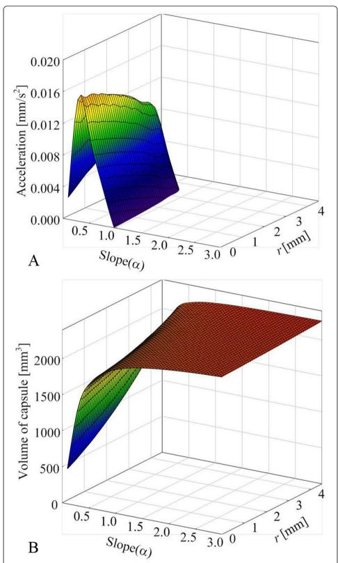
**Figure 9 Exterior shape simulation results**. (a) Relationship between acceleration and shape of the capsule. (b) Relationship between volume and shape of the capsule.
