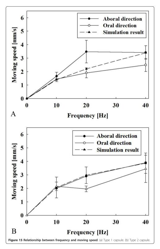
moving speed of the capsule is proportional to the frequency, the frequency parameter can be used to control the moving speed of the capsule.
