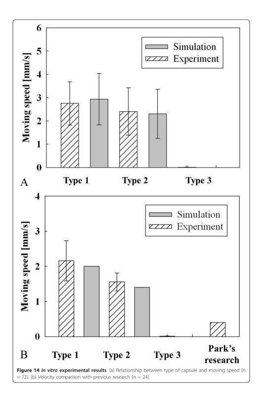
stimulation results from current experiment (6 V, 10 Hz, 5 ms) data were compared. Even though the total energy applied to the small intestine was 10 times lower than previous studies, the average moving speed of current experiments was 5.2 times faster than the previous research.
