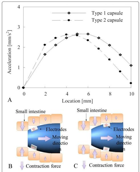
**Figure 11 Electrode position simulation**. (a) Relationship between location and acceleration. (b) Illustration of moving capsule when electrodes are placed at the left edge of the capsule. (c) Illustration of moving capsule when electrodes are located a bit to the right of the left edge of the capsule.
