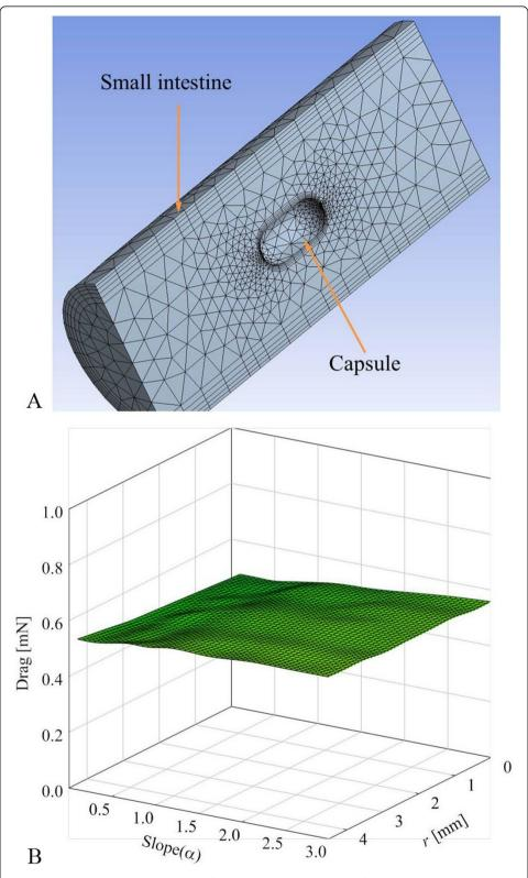
**Figure 6 Drag depends on the shape of the capsule**. (a) Illustration of finite simulation with meshes. (b) Drag depends on various shapes of the capsule at fixed velocity (0.5 mm/s).
