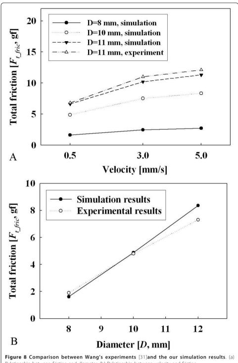
Relationship between friction and diameter. (b) Relationship between velocity and friction.
