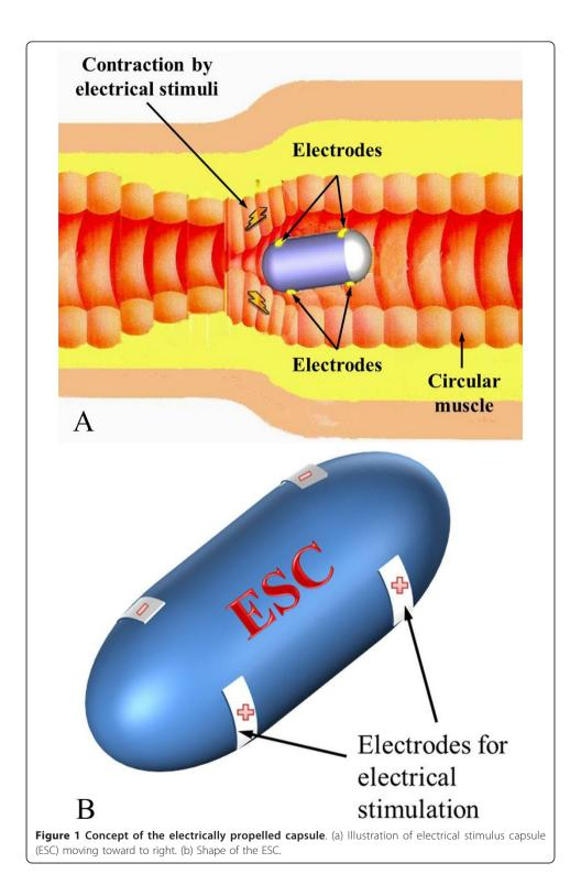
In order to move the capsule, the contraction force of the small intestine causes it to move the capsule, as shown in Figure 2. It is assumed that the capsule is moving to the right and small intestine is contracted by electrical stimuli. Since the capsule is moving toward the right, the left part of the small intestine is stimulated for a long time and causes large contraction force. The small intestine is composed of smooth
