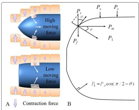
**Figure 5 Capsule shape and moving speed**. (a) Illustration of faster velocity of streamlined capsule compared to cylindrical capsule. (b) Mathematical relationship between the shape of the capsule and moving force.
