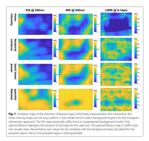
In the case of movement in the adult and baby measurement, some maps show lower values in  $ROI_{pulse}$  compared to  $ROI_{BG}$  for VIS (e.g., *band power* according to Tables 1 and 2).
