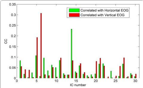
**Figure 7 Correlation coefficients between EOG activities and independent components (ICs)**. This figure shows the correlation coefficients (CCs) between the ICs and EOG in horizontal and vertical direction respectively.
