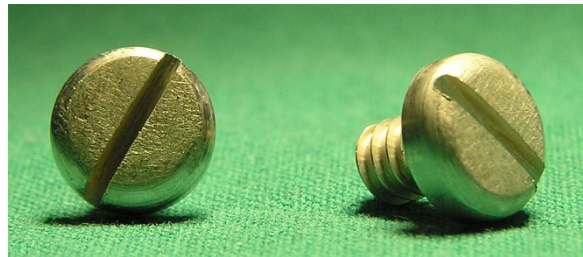
Figure 1 MgCa0.8 bone screws, which were implanted into rabbit tibiae. The slotted screw head had diameter of 8.0 mm.
