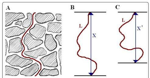
**Figure 3 Determination of tortuosity through a porous material using the arc-chord ratio**. The tortuosity of a path through a porous structure (A) can be determined by the ratio of the pore length, L, to the displacement, X. As can be seen in (B) and (C), the magnitude of L remains constant but as the compression increases the displacement X reduces to X' which results in an increase in tortuosity.
