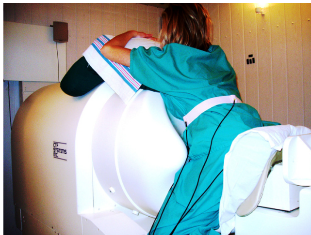
Figure 1 SARA system for measurement of the magnetic activity of the uterine. (Courtesy of CTF Corporation.)
