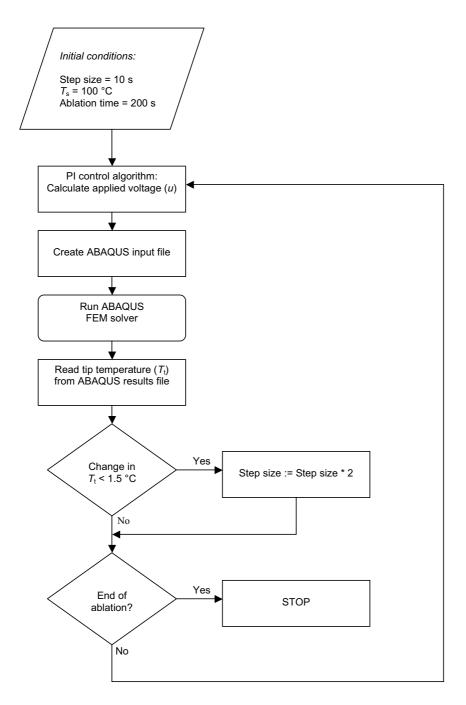
**Figure 6** Flowchart of the control software implementing a PI control algorithm.
