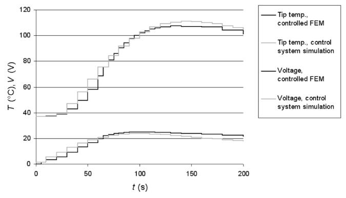
**Figure 4**Temporal behavior of tip temperature and applied voltage of the closed loop system. The upper curves show the tip temperature, the lower curves show the applied voltage. The light curves show the results of the control system simulation. The dark curves show the results of the FEM model controlled by the control software.
