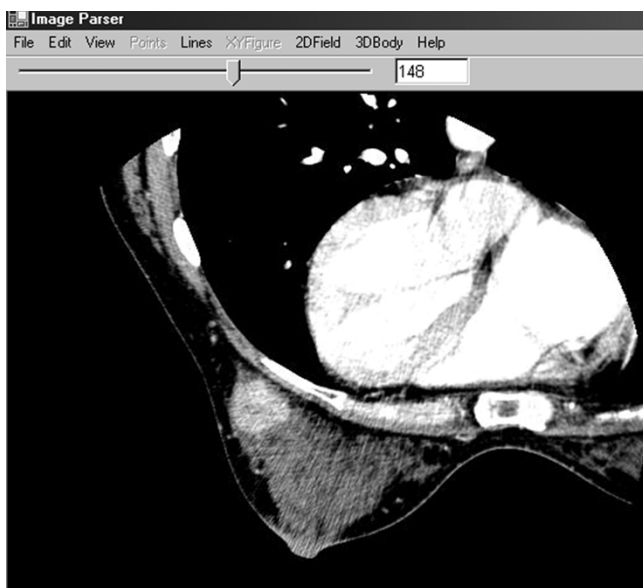
Figure 1 The Interface of ImageParser When Loading a 3D Image. The image is automatically shown slice by slice with the slice number shown in the text box, and the interval between two slices can be changed. Clicking the slide bar or text box, we can focus on the current slice; double clicking the window area, we can navigate the image slice by slice again; and dragging the slide bar or inputting the slice number in the text box, we can jump to the desired slice.
