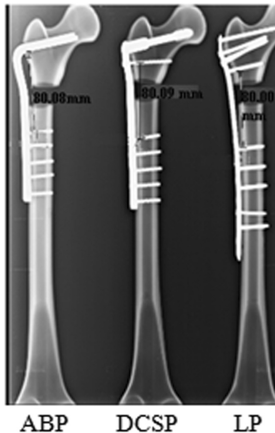
Figure 3 Working lengths as measured on the radiographic images of the composite constructs of SFF fixed with the three implants.
